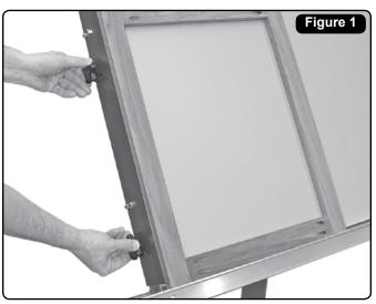
Place workpiece into alignment with squaring fence
