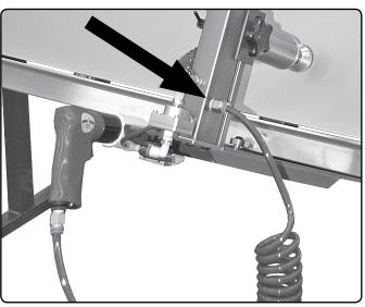
Fitting where screw gun is connected to the table.
