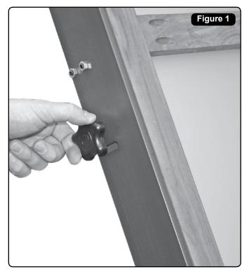
Loosen locking knobs on side of fence
