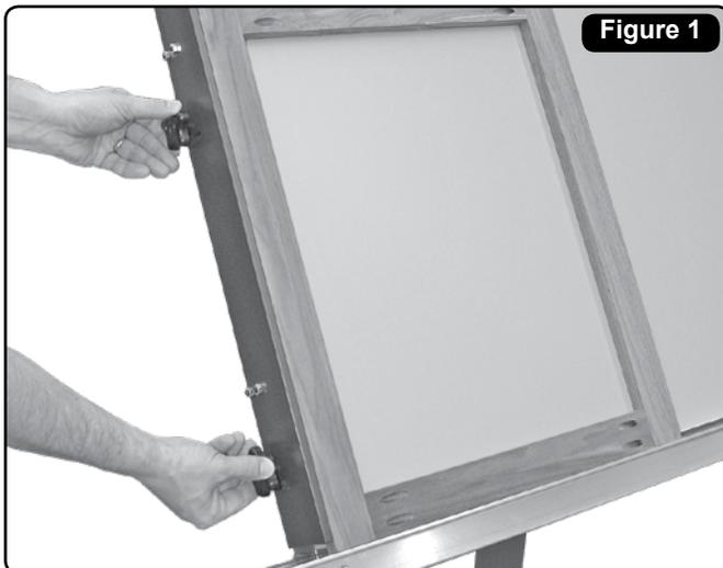
Place workpiece into alignment with squaring fence
