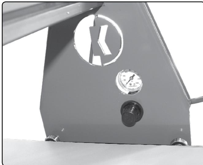
Regulator controls amount of air pressure to the screw gun.
