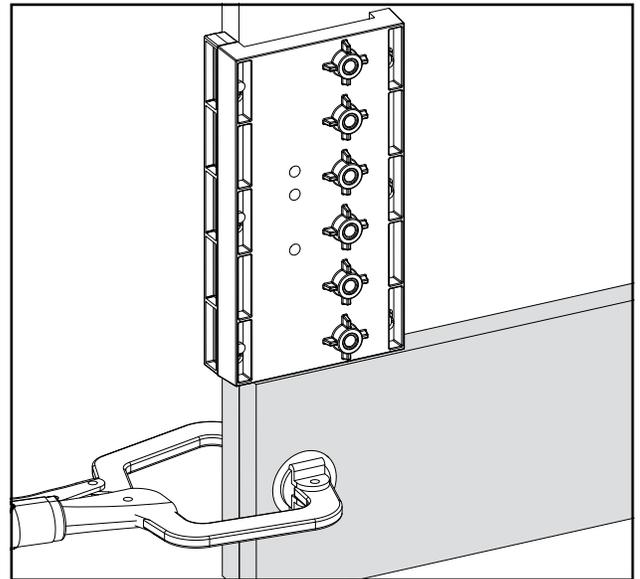
Sometimes you don't need a continuous column of holes spaced every 1 1/4" [32mm] on centre. To skip holes without losing alignment, follow the instructions in the section Using the indexing pin, but after repositioning the jig, skip four holes and drill only the last shelf-pin hole. Now reposition the jig with the indexing pin inserted in this single hole and drill the remaining five holes. Repeat as necessary.
