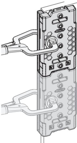
**Tip** If your cabinet is already assembled, remove the fence and place the jig against the back of the cabinet using the same reference point as the front and carefully hold in place while you drill your first hole. Then use the jig extender and index pin to continue.
