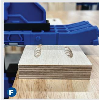
**A** Optional: Workpiece edges and pocket holes can be sanded prior to assembly.
