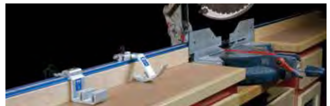
Place 6 feet (1830mm) of Trak on one side and 2 feet (610mm) on the other side.
