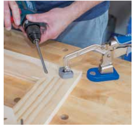
Bench Clamp keeps pieces perfectly aligned to create tight-fitting joints.
