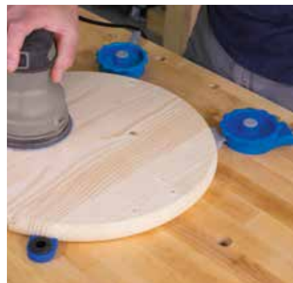
Clamp shoe holds flat and rounded shapes, as well as 90°.
