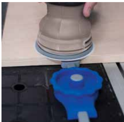
Low-profile design keeps clamp out of the way while working.
