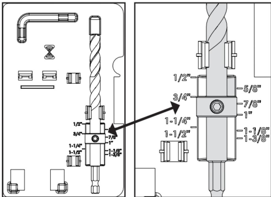
**The example shows the stop collar positioned for a  $\frac{3}{4}$ " (19mm)-thick workpiece.**
