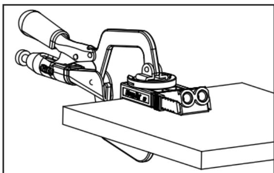
With the included clamp pad adapter, the Kreg Jig® R3 can be connected to any Kreg face clamp for faster positioning and clamping.
