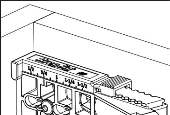
In situations where it is not possible to clamp the jig in place, secure the jig to the workpiece by driving a wood screw through the mounting hole. Remember to position the drill-bit stop collar to match the thickness of your workpiece.
