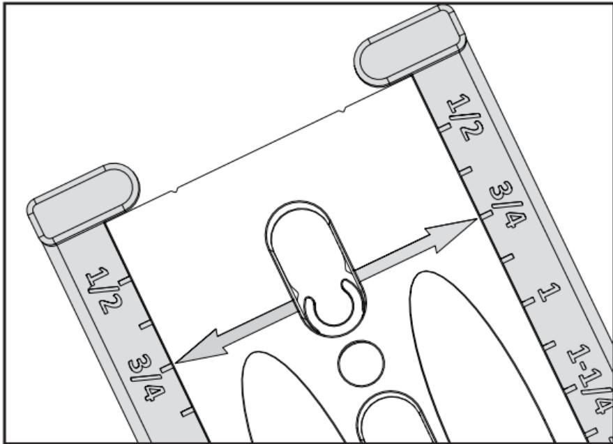
**The example shows the sliders positioned for a  $\frac{3}{4}$ " (19mm)-thick workpiece.**
