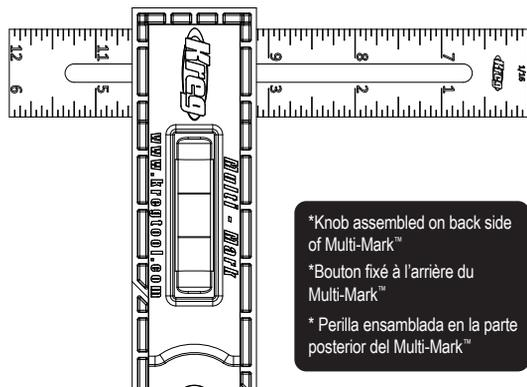
The Multi-Mark™'s second position sets the scale at a 90° angle. This is good for squaring your projects and making marks at a 90° angle.
