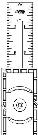
The Multi-Mark™'s third position sets the scale at a 0° angle, in line with the base. This is good for use as a depth gauge on your table saw as well as a general scribing tool or simply transferring measurements.
