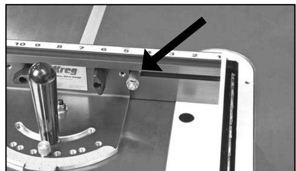
Position Stop installed.
