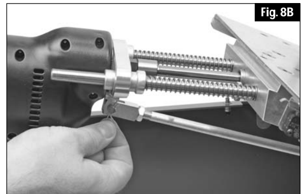
Disconnect the Connecting Rod to remove the Electric Drill Motor from the Guide Rods.
