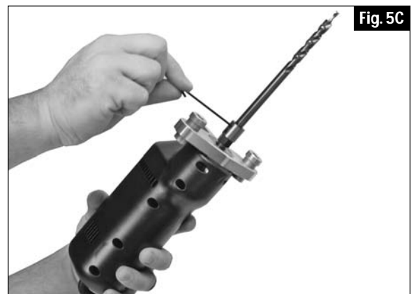
The Drill Bit is held in position with set-screws in the Drill Adapter.
