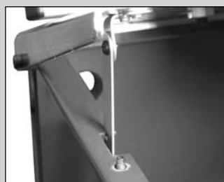
This latch will automatically catch and hold assembly in place.
