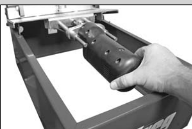
Push motor in slightly and lift assembly up until latch catches on left side of machine.
