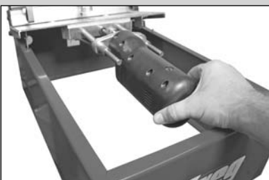
Push motor in and lift assembly up until latch catches on left of machine.
