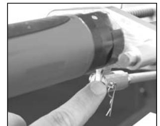
Removing Clevis and Cotter Pin from the Connecting Rod.
