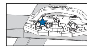
End of Board (obstructed) When securing the end of a <sup>3</sup>⁄4"- to 1 1/8"-thick deck board with a 2"-long Kreg Deck Screw where the Deck Jig™ cannot protrude beyond the end of the board (wall obstruction), align the end of the jig with the end of the board and use the End Drill Guide.
